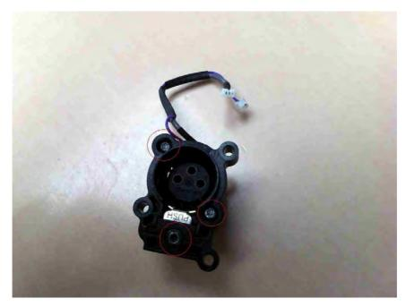
Turn over the XLR. Undo and remove the two T8 torx screws and the 3mm Alan bolt
